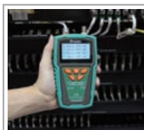
Locate break point and length measurement
