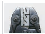
Interchangeable die with quick release trigger
