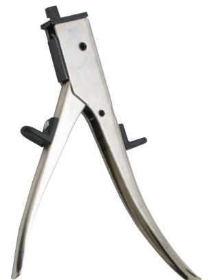
A scribe line can be followed by locking down on work in this position. A slot is cut by making successive cuts.
