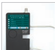
RJ11/12 telephone wire test
