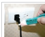
Red LED and audible alarm if voltage is present
