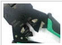
Stripping twisted pair round cable
