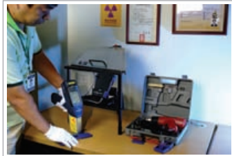
Handheld XRF for RoHS Compliance Testing
