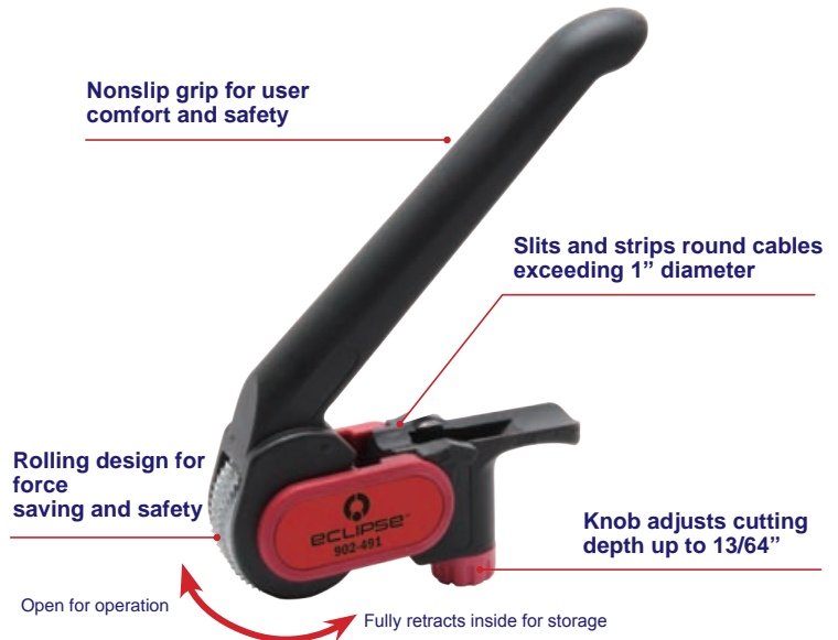
Adjustable cutting depth
