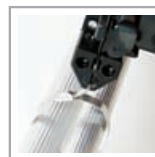
Tensioning and cutting off stainless steel cable ties
