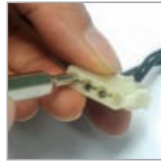
Put the pin extractor into housing
