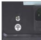
Additional ground contact
