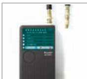
BNC coaxial cable test
